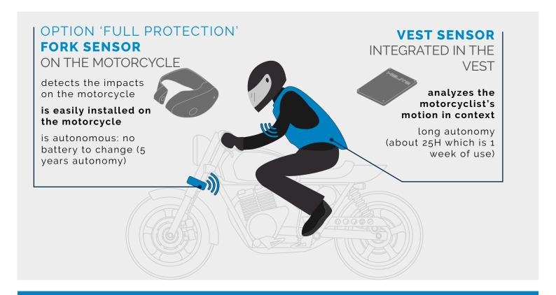
Detection time of the airbag vest (CDU sensor): 60 ms / with fork sensor: 31 ms
